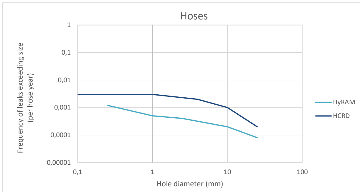
Figure 6-8 Hose leak frequency relative to hole diameter (Source: DNV).
