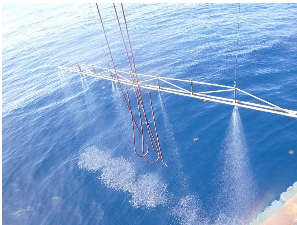
Figure 2: Quarterly drill on board Adelia . Dispersant spraying system test
