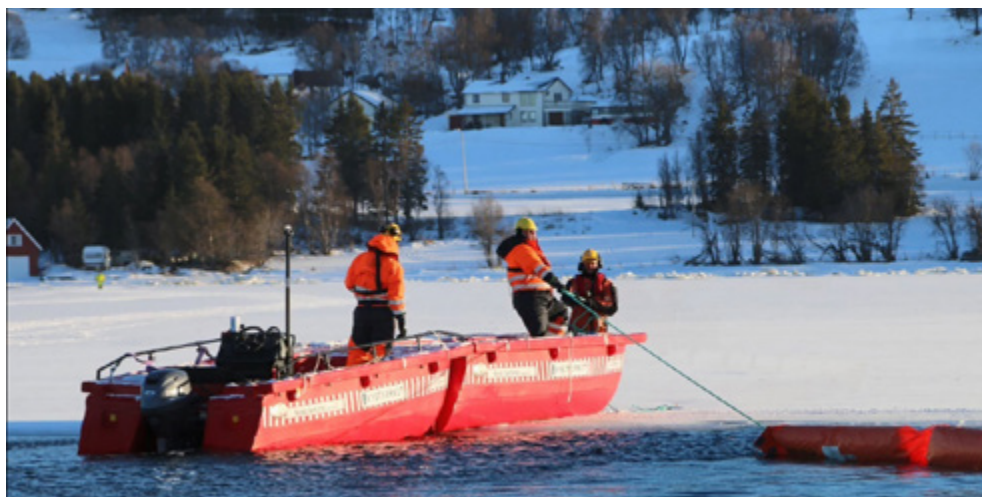
From a winter training course in northern Norway. Here the boom is attached with an ice screw to the ice. Personnel on the ice has a survival suit and safety line in case the ice breaks. Picture: Tor-Åge Thomassen, NCA.
