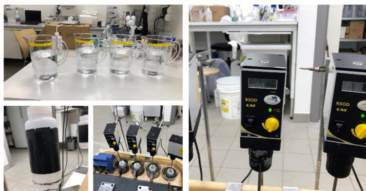
Figure 15. From left to right, from up do down: The release rate measuring tanks; the rotating device for biocide extraction at 60 rpm; the cylinder painted on a 200\text{cm}^2 area and the extraction moment in the water bath at 25^{\circ}\text{C} \pm 1^{\circ}\text{C} .
