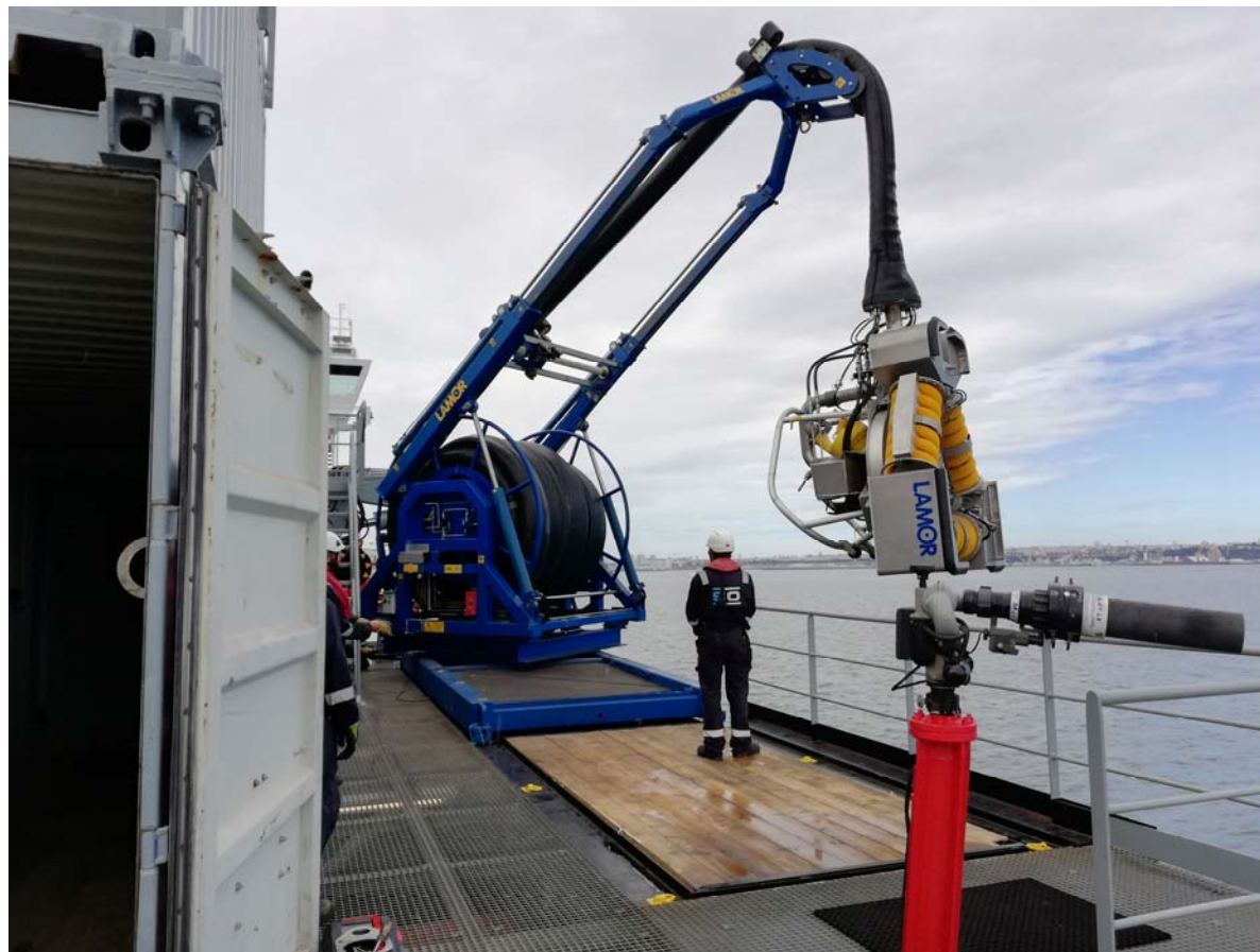
Fig. 1 Acceptance drill on board VN Partisan. High capacity skimmer test.
