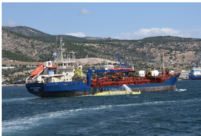
Fig.7. Aktea OSRV collecting oil with sweeping arm system
