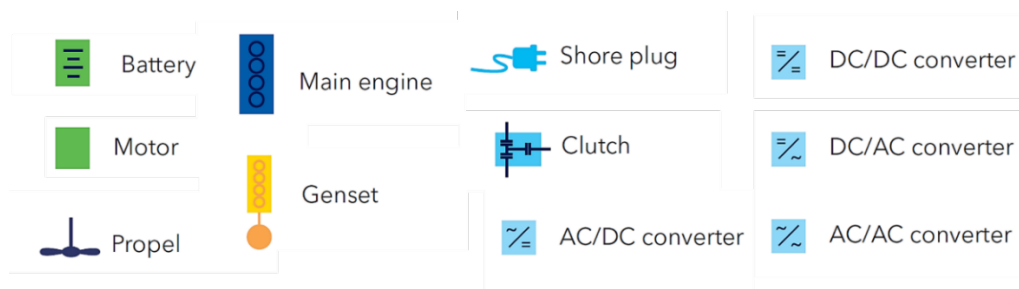
Figure 3-2 Systems for electric components used to build different topologies where maritime batteries are integrated
