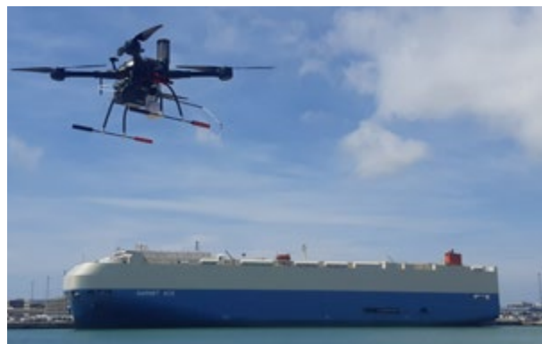
RPAS equipped with gas sensors can take measurements of air emissions from ships
