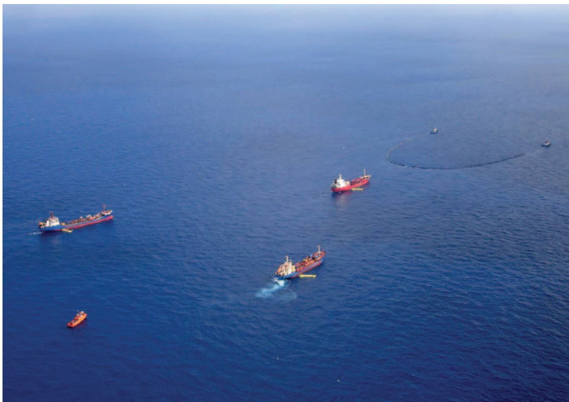
Mistra Bay, Aktea OSRV and Santa Maria simulating the collection of oil behind the "Open U" boom configuration during Exercise Malta 2008
